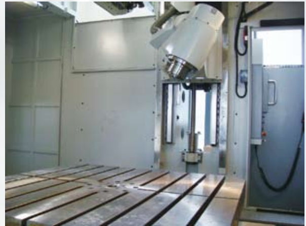
B axis swivel head at tilting angle position.
