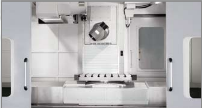
1200 x 1200mm CNC rotary table built in on EBM-2150
