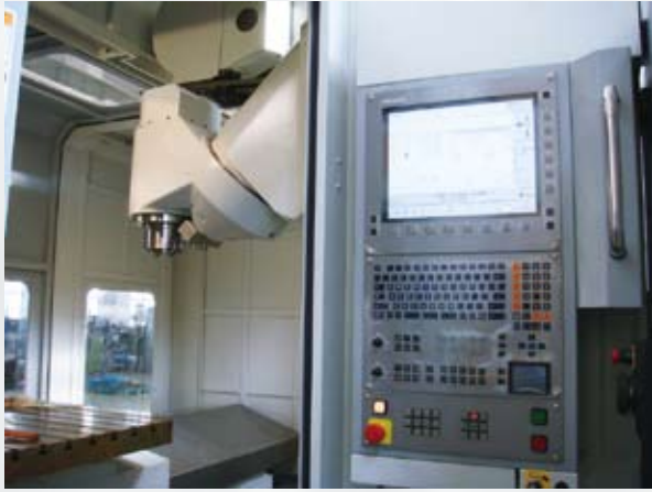
B axis swivel head at vertical position.
