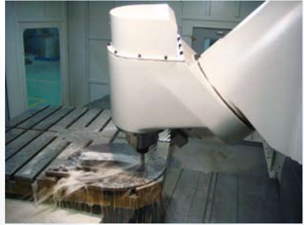
B axis swivel head at vertical position.
