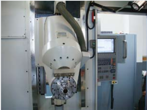
B axis swivel head at tilting angle position.
