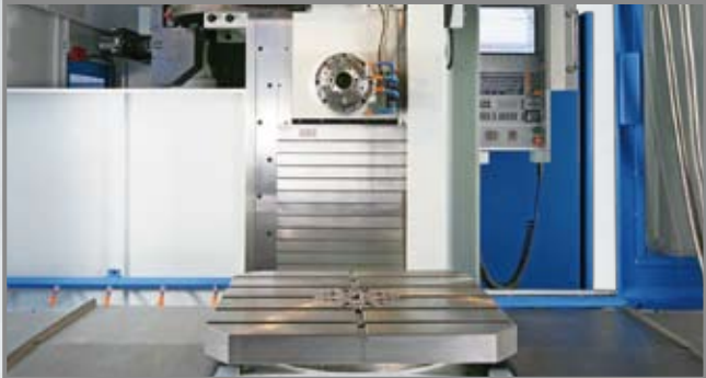
700 x 800mm CNC rotary table built in on EBM-1000
